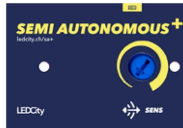
The radar sensitivity can be adjusted with the rotary knob on the backside of the sensor head.
